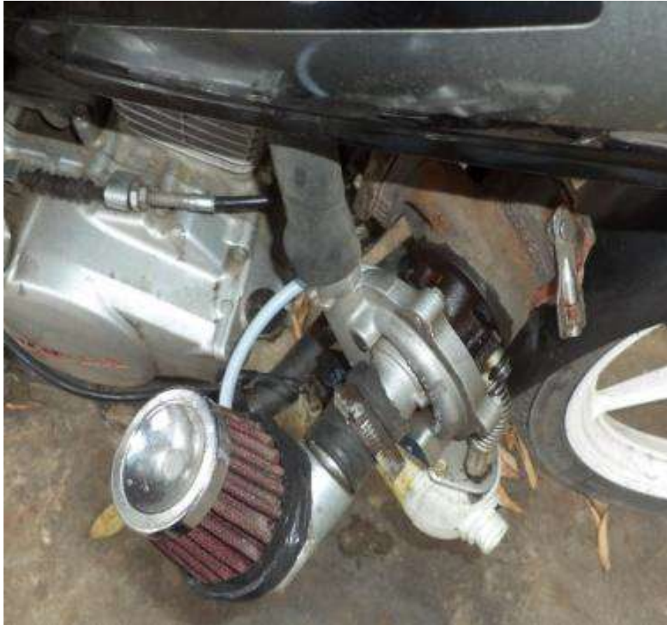
Figure: Installed Turbocharger
